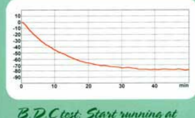
B.D.C test: Start running at constant speed Press start continuous running. The maximum gap is 0.08mm. The B.D.C. keeps stable after 30 minutes during running continuously.
